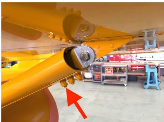
3. Ensure the wing is properly supported and then remove the strut-wing mounting bolt. These are usually installed from the front, towards the back.
