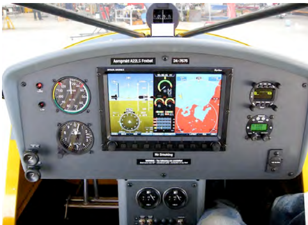
Dynon 10” SkyView – the screen can be configured to show any one or more of flight instruments, engine parameters and GPS
