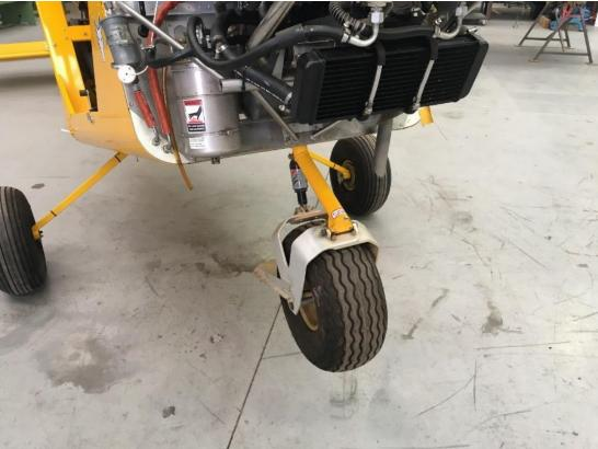
2. Make sure that the bolt in not seized by applying light pressure using the appropriate size spanner first, before removing it. If the bolt was seized, it is likely that large forces were exerted on the lower attachment bracket and therefore, must be inspected thoroughly for cracks and over stress damage.
