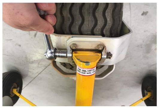
3. Remove the split pin, nut and bolt and carefully lower the leg and wheel to the rear.
