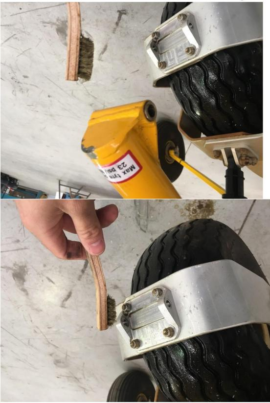
5. Once the parts are cleaned, perform a detailed inspection on the bracket and all attachment points, as well as the nose leg itself.
