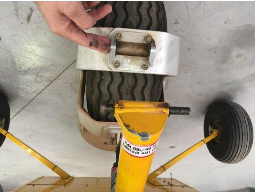
4. Clean the area using anti corrosive products and use a soft tool to agitate all dust and remove older grease deposit off the bracket and bolt, be careful not to damage the bronze bushes on either side of the nose leg.
