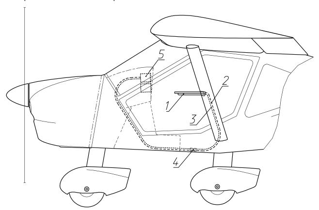
Fig. 10 Full and static pressure system
