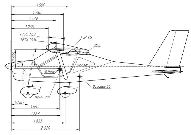
Fig. 1 CG location of the empty airplane, pilots, fuel and baggage
