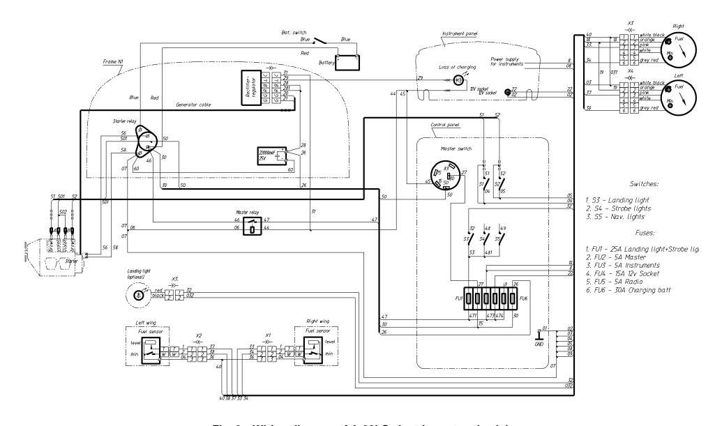
Fig. 3 Wiring diagram of A-22LS electric system (main)
