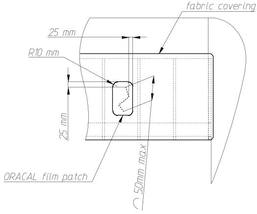
Fig. 12 Fabric covering repair
