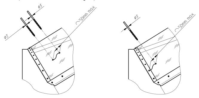
Fig. 11 Fuselage glass crack stop-drilling
