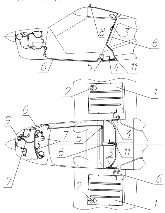
Fig. 2 Fuel system schematic
