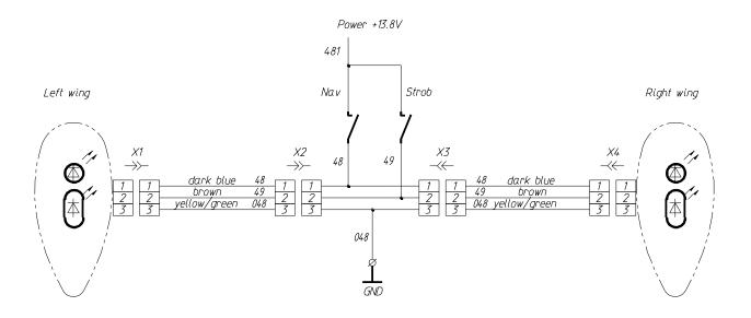
Fig. 8. Wiring diagram for installation of strobes
