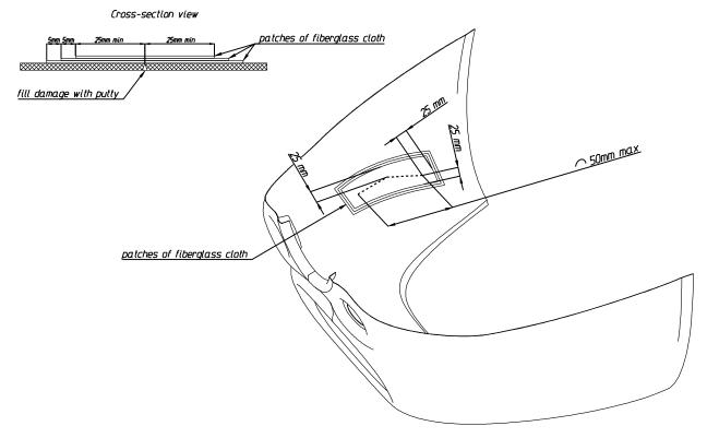
Fig. 13 Composite parts repair
