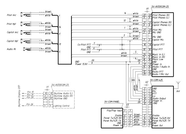
Fig. 6 Wiring diagram for Dynon SkyView radio
