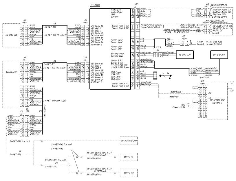
Fig. 5. Wiring diagram for installation of SV-D1000, SV-GPS-250, SV-BAT-320, SV-ADAHRS-200
