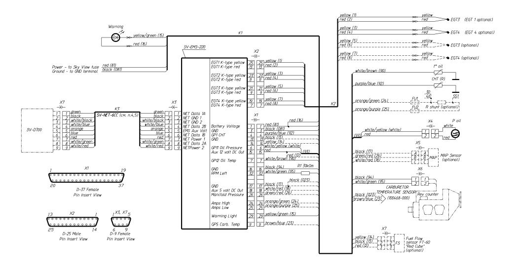
Fig. 4. Wiring diagram for installation of SV-EMS-220
