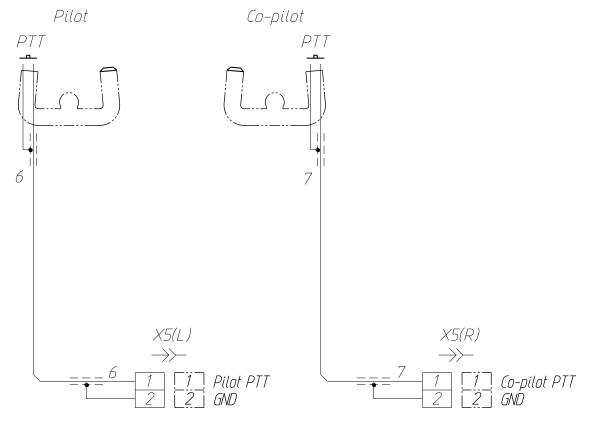
Fig. 7. Wiring diagram for installation of PTT and trimmer control button
