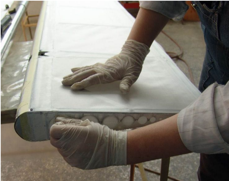
Photo 33 (at end ribs the fabric may be pressed down using a towel)
