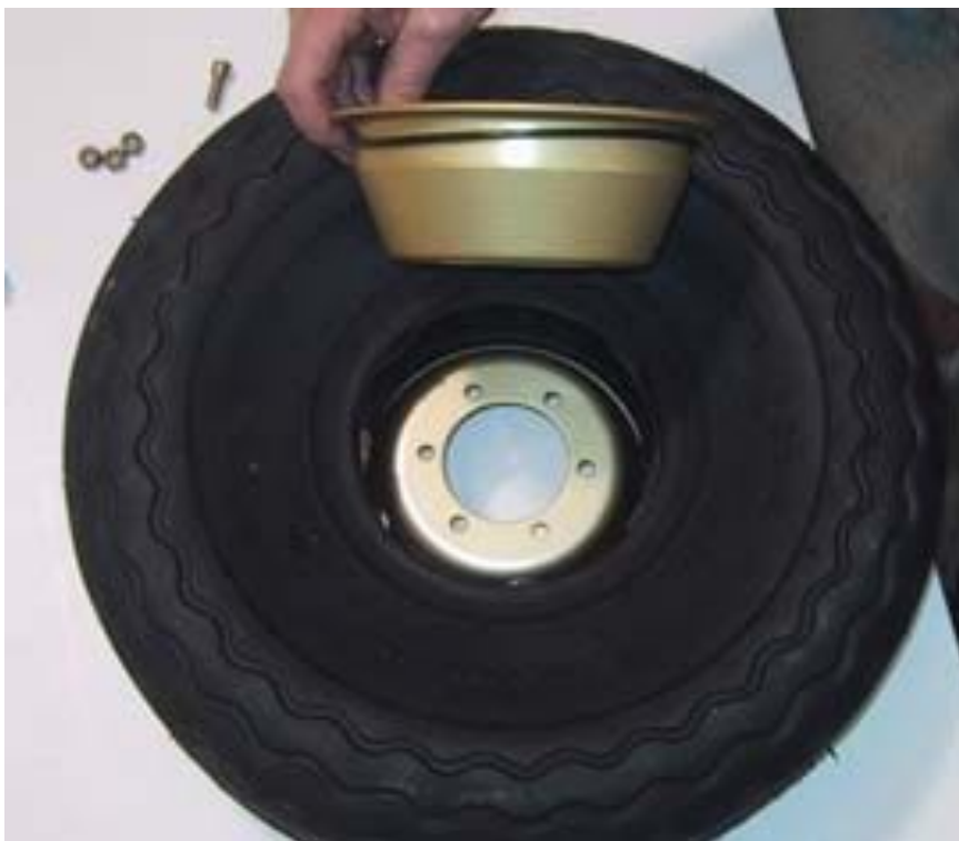
5 Insert wheel half with o-ring into tire and mate with opposite half. O-ring is still installed on bead seat.
