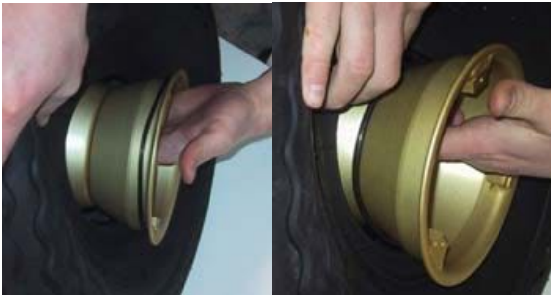
7 Compress tire side walls slightly and slide o-ring into groove between wheel halves.
