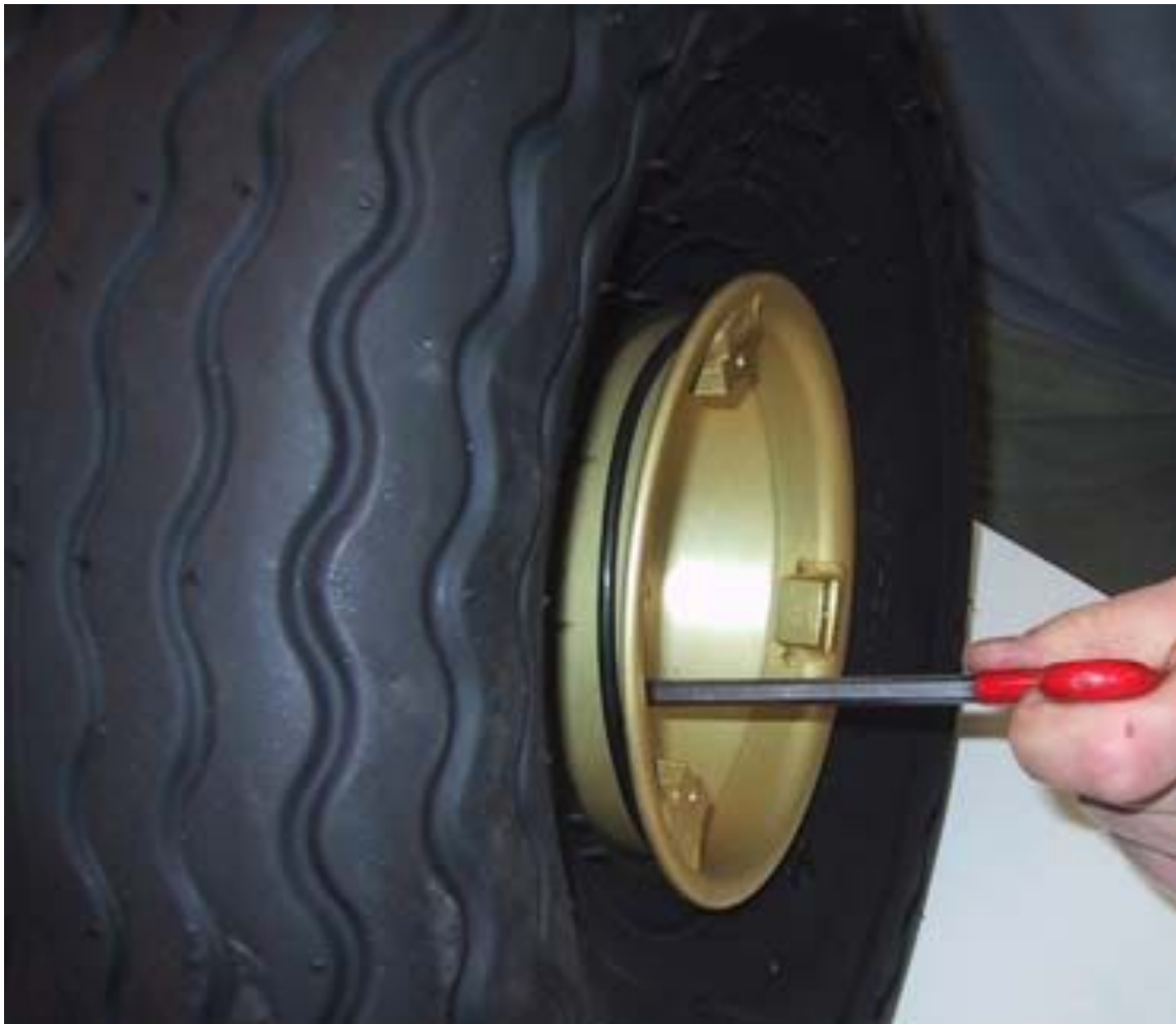
6 Bolt wheel halves together with .31-18x.875 bolts installed in every other bolt hole.
