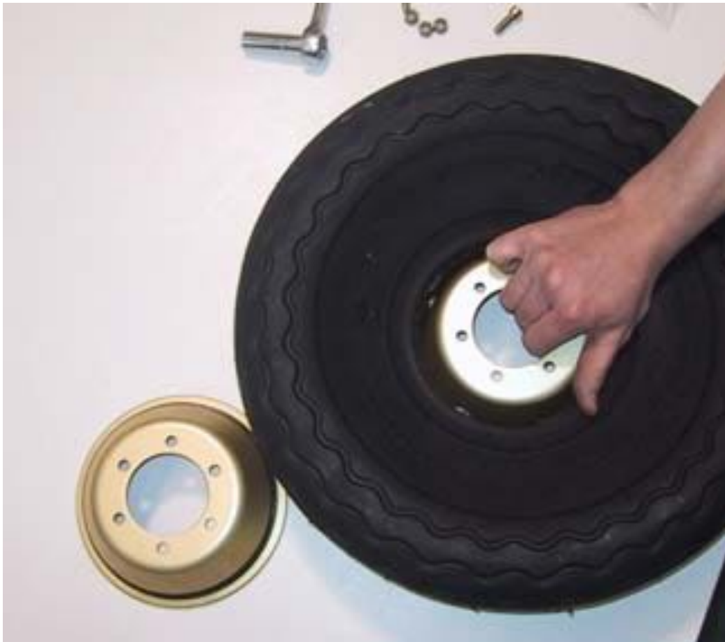
4 Insert the other wheel half into the tire
